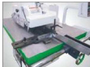
短料装置, 最短可加工200mm。 Short workpiece machining unit: Min 200mm in continuous material feeding
