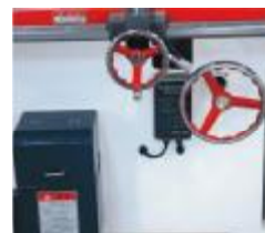
主轴可升降技术，根据加工厚度实际，自由调整锯片高度。 Saw spindle can be adjusted freely according to the working thickness.
