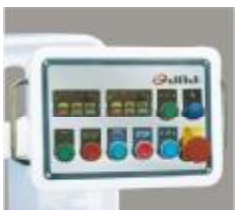
送料变频控制，快达40米每分钟 Inverter controlling feed system, up to 40m/min
