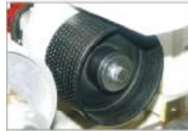
钉状压轮，适用于锯材加工。 Spine pressure wheels, suitable for sawn timber processing.
