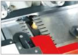
特殊处理的超耐磨唇板。 Slotted table plate wear-resistance treated.
