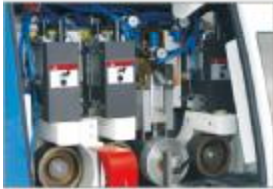
上驱动式重型进料压辊，可加工弯曲木材。 Positive pressure wheels, suitable for bent material processing
